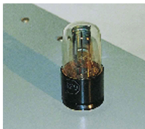
Figure 29.7 The photoelectric effect can be observed by allowing light to fall on the metal plate in this evacuated tube. Electrons ejected by the light are collected on the collector wire and measured as a current. A retarding voltage between the collector wire and plate can then be adjusted so as to determine the energy of the ejected electrons. For example, if it is sufficiently negative, no electrons will reach the wire.
